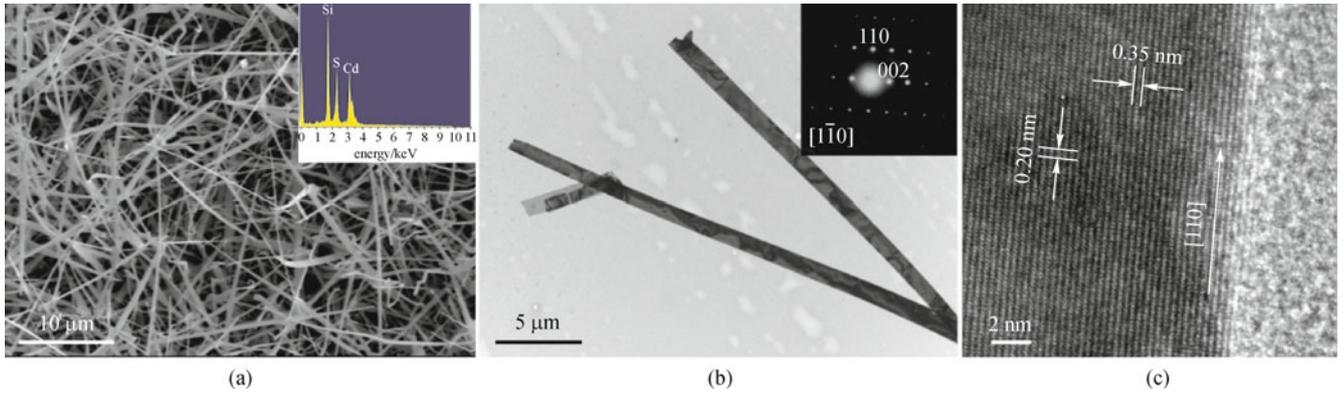
**Fig. 2** Morphologies and structures of CdS:Ag NRs. (a) Typical FE-SEM image (inset shows EDS spectrum); (b) low-resolution TEM image (inset shows corresponding SAED pattern); (c) HRTEM image
