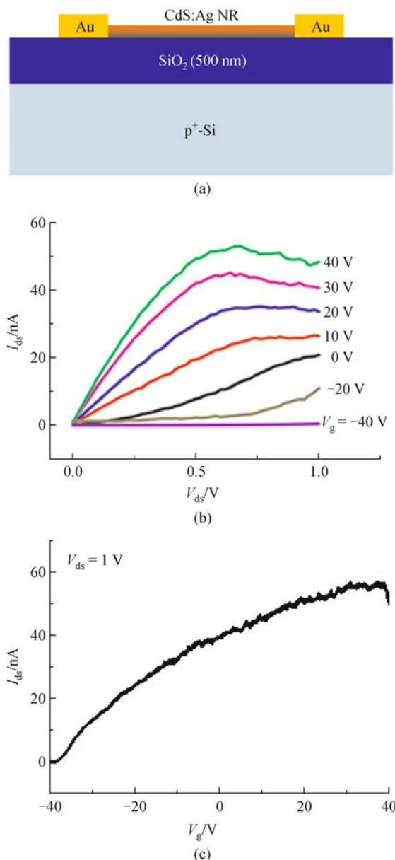
**Fig. 4** Transport characteristics of back-gate nano-FET based on CdS:Ag NR. (a) Schematic illustration; (b)  $I_{\text{ds}}-V_{\text{ds}}$  curves measured at varied  $V_{\text{g}}$  ( $V_{\text{g}}$  increases from 0 to 40 V in a step of 10 V); (c)  $I_{\text{ds}}-V_{\text{g}}$  curve at  $V_{\text{ds}}=1 \text{ V}$
