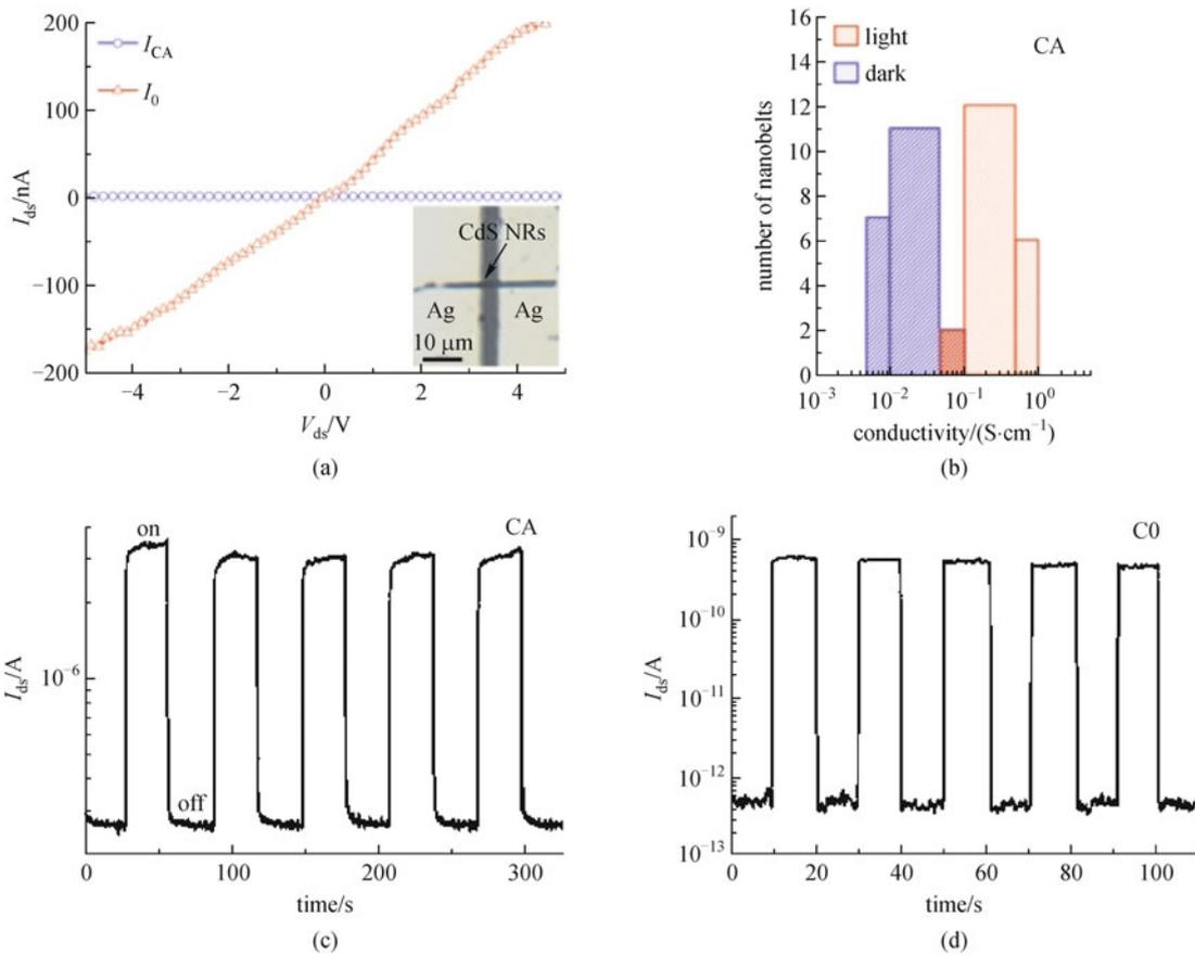
**Fig. 3** Electrical and photoconductive properties of CdS:Ag NRs. (a) Typical  $I_{ds}$ - $V_{ds}$  curves of CdS NRs (doped and intrinsic) in dark (inset shows photo of typical device based on single CdS:Ag NRs); (b) conductivity distribution of 20 CdS:Ag NRs in dark and upon light illumination; (c) time response of sample CA; (d) time response of sample C0 (LED white light from microscopy was turn on/off manually;  $V_{ds}$  was fixed at 5 V)
