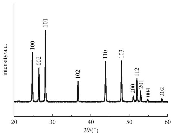
Fig. 1 XRD pattern of as-prepared CdS:Ag NRs
