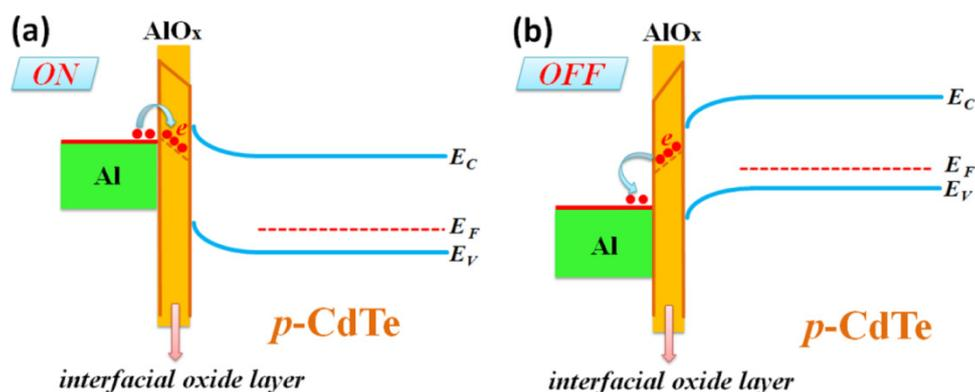
**Figure 6.** (a) Schematic energy band diagram for the Al/CdTe:Sb Schottky junction in the ON state when a forward bias is applied to the Cu/Au electrode. The electrons are trapped in the interface states. (b) Schematic energy band diagram for the device in the OFF state when a reverse bias is applied to the Cu/Au electrode. The trapped electrons are released to the Al.
