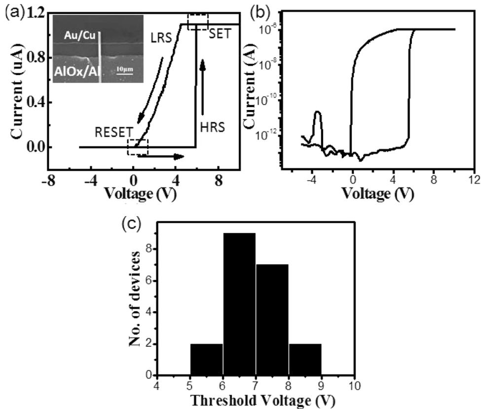
**Figure 2.** (a) Switching characteristics of the Al/AIO<sub>x</sub>/CdTe:Sb NW junction, where the LRS and HRS indicate the low and high conduction states as the ON and OFF states, respectively. The inset is a typical FESEM image of the memory device. Note that the Au/Cu electrode was grounded during analysis. (b) The semi-log plot of the hysteresis behavior. (c) Statistical distribution of the threshold voltage of 20 devices.
