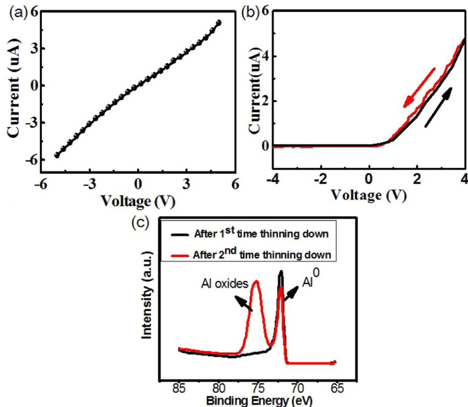
**Figure 5.** (a)  $I$ - $V$  curve of an Sb doped CdTe NW with two Cu/Au electrodes on both ends. (b) The typical  $I$ - $V$  curve of the Al/CdTe:Sb NW Schottky junction with a dual sweep. (c) XPS spectra for Al peaks at high resolution.
