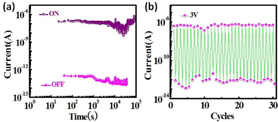
**Figure 3.** (a) Retention characteristics of memory device measured at  $V = 3$  V; the device was switched ON using +10 V, and was switched OFF using -10 V. (b) Bistable resistance for the HRS and LRS as a function of switching cycles.
