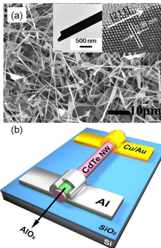
**Figure 1.** (a) SEM image of the as-synthesized CdTe:Sb NW, the left inset is a TEM image of an individual Sb doped CdTe NW, the right inset shows the corresponding HRTEM image. (b) Schematic illustration of a nonvolatile memory device based on Al/AIO<sub>x</sub>/CdTe:Sb NW.
